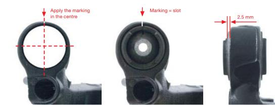
The slot in the new rubber mount must be aligned with the marking on the trailing arm, then installed with a suitable special tool until the mounting is pressed in, up to the dimension of 2.5 mm.
